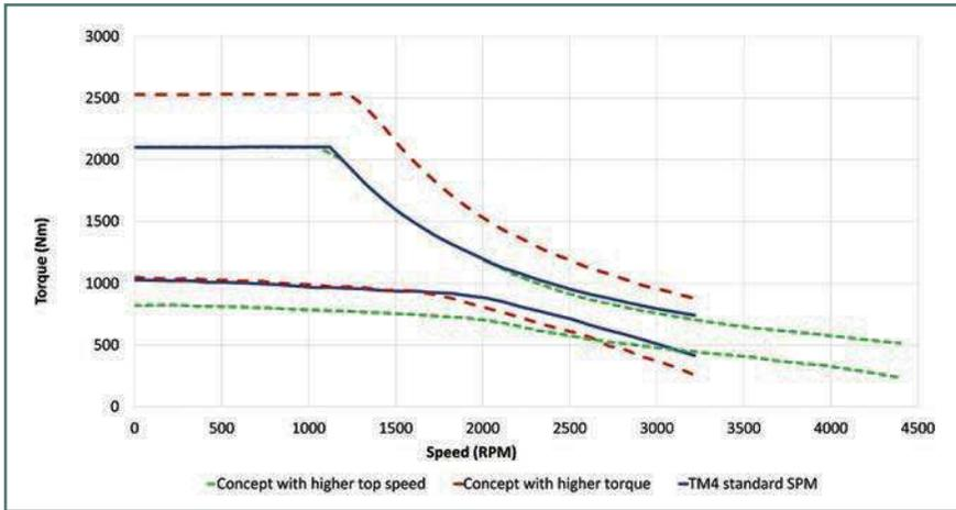
Figure 2: A performance comparison of the permanent magnet motor using the new reluctance-assisted outer rotor technology, and the original surface-mounted machine
