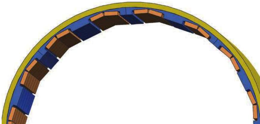
Figure 1: A strip of lamination added to the rigid carbon still rotor satisfies saliency and rigidity requirements
