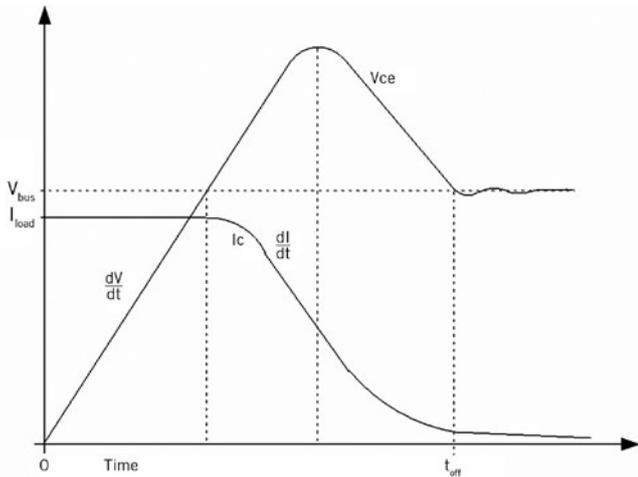
② Shape of the voltage and current across the IGBT at turn-off
