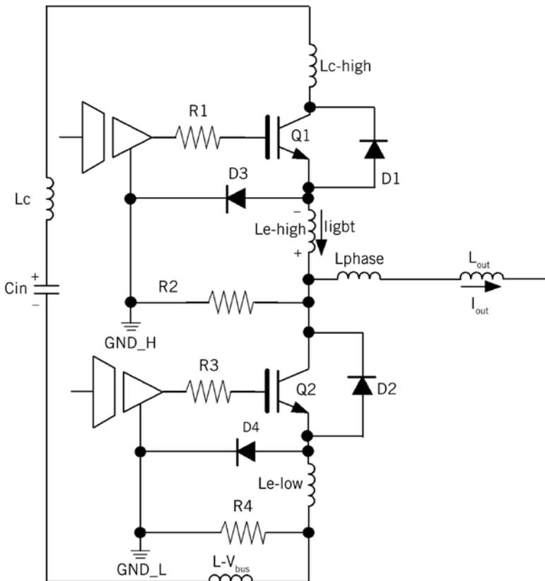
④ Equivalent circuit of the IGBT module and the inductances of the connections
