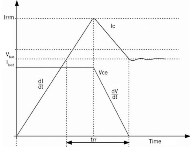
③ Shape of the voltage and current across the IGBTs at turn-on
