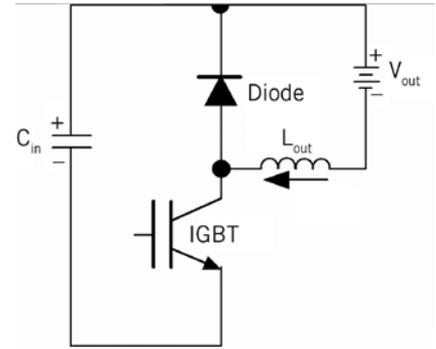
❶ Equivalent circuit of a commutation cell
