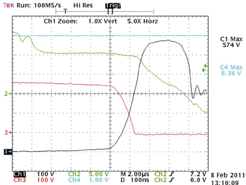
9 Turn-in in short-circuit condition with a bus voltage of 350 V
