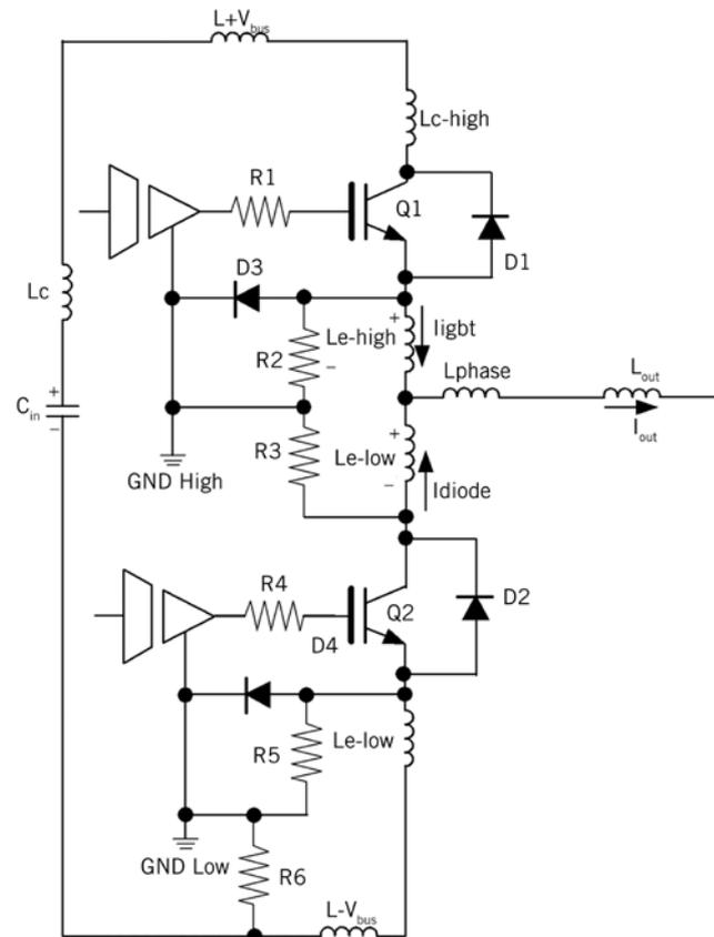
6 The resistor divider is limiting the effect of the emitter inductance
