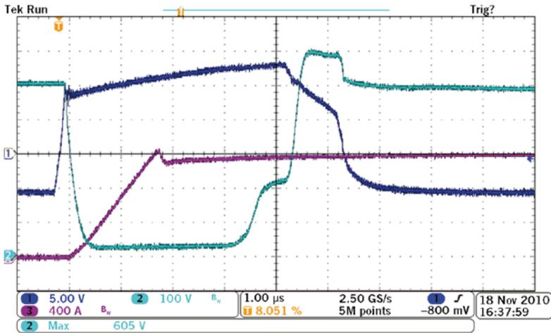
5 Turn-off using the stray inductance to limit the overvoltage
