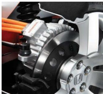
The 2006 Honda FCX has three electric motors: one front-drive motor with an output of up to 108ps, and two smaller motors with a maximum output of 34ps driving each of the rear wheels
