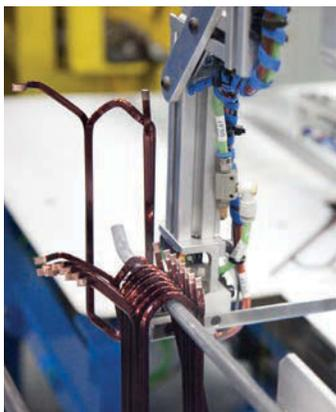
Patented wire coil forming machine used during the stator manufacturing process at TM4's Boucherville facility
